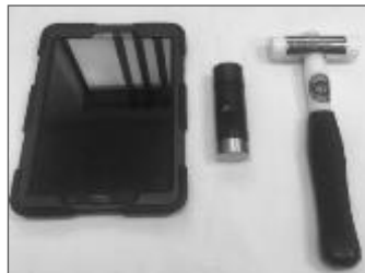
Figure 3. Fieldwork component (Computerized hand-held device, sensor and hammer)
